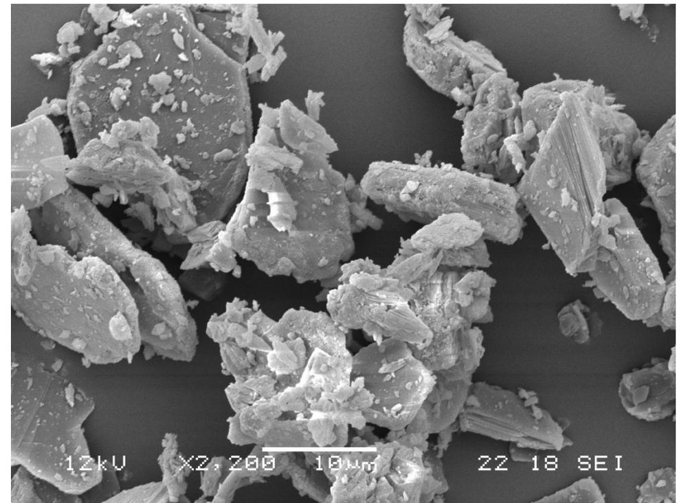
**⇒ Due to low decomposition temperature, ATH not suitable for most of PP compounds**
