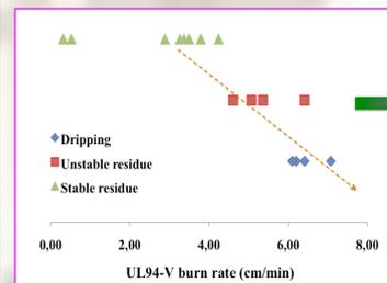
Fig. 4 - Correlation between the formulations residue behaviour during DIN 4102 test and the burn rate in UL94 vertical test.
