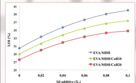
Fig. 2 - LOI regression model as a function of Sil amount at different CaB percentages.
