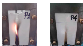
Figure 2. Vertical burning test of EVA-compounds with MDH alone (P1) and boehmite (P4).
